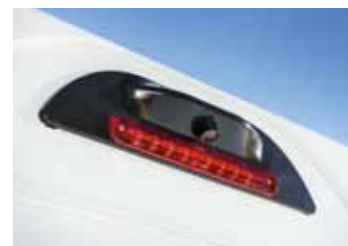
Backup camera built into the rear band with a screen on the rearview mirror.
