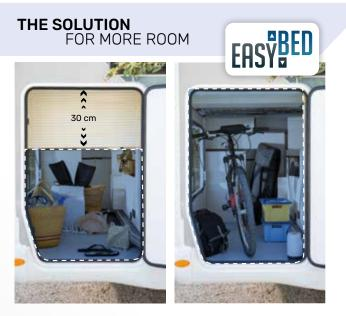
The EasyBed system lets you raise or lower the bed to adjust the size of the hold area according to your needs.
