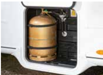
Low load sill to simplify gas bottles change.
