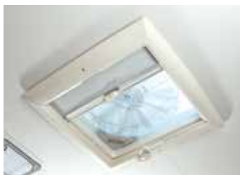
The ventilator/extractor skylight** , allows extracting stale air and ventilating the inside very quickly.
