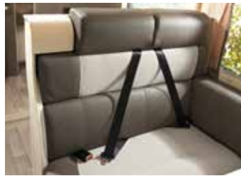
Seat belts corresponding to the number of regulation seats; at least four belts with three points.
