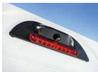
Backup camera built into the rear band with a screen on the rearview mirror.
